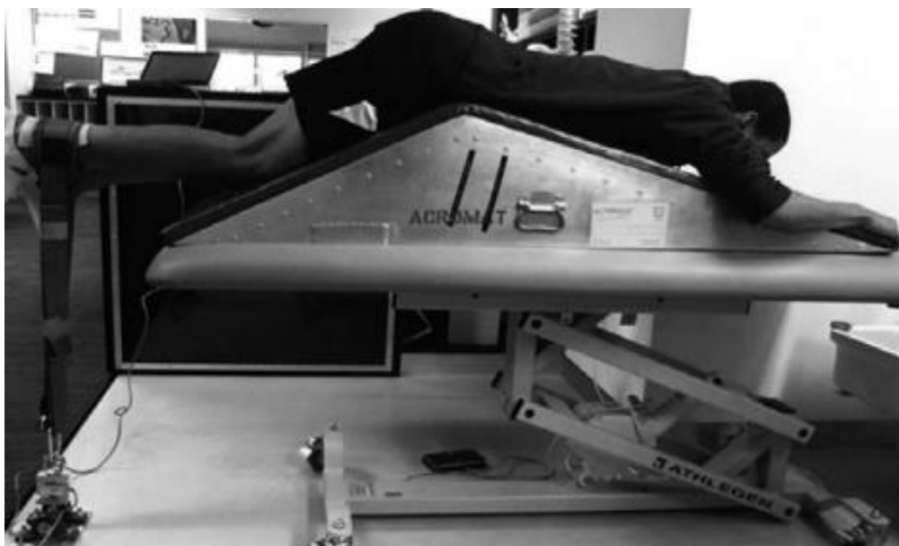
FIGURA 5 – MESA FLEXORA ISOMÉTRICA (WOLLIN ET AL., 2017)
