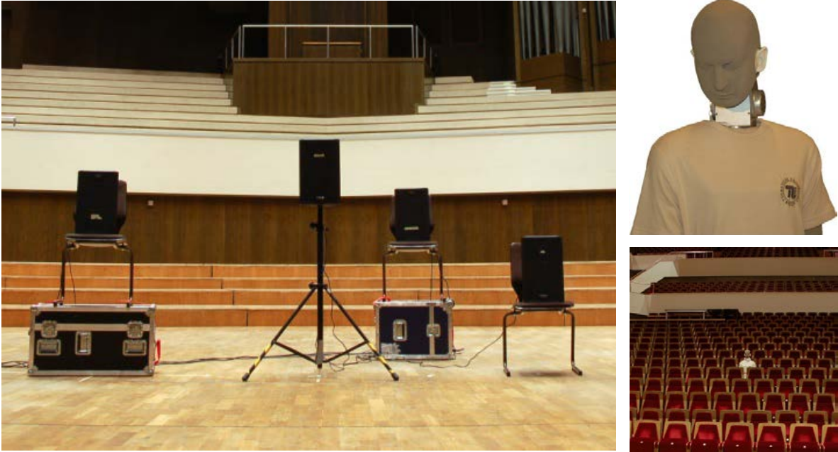
Figure 3: Playback of excitation signals and recording of binaural room impulse responses using the head and torso simulator FABIAN .
