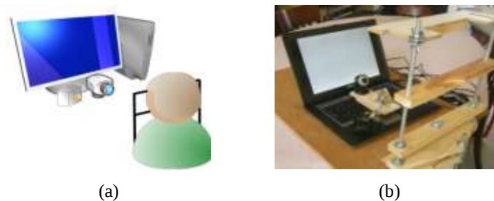
Figure 1. (a) Overview of the hardware design. Note that the camera and the infrared light source are placed near the computer screen. (b) A picture of the real setup.
