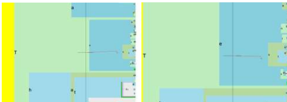
Figure 9. Example of the usage of the Dasher software for typing the word “Test”. In this example the user already selected the character T, and aims toward the letters e and s. The second figure is one instance later when the program zoomed into the region of interest and the character e is already selected. The software varies the size of the boxes of the characters based on the probability that a character can occur. For this example the probability of the character “s” after the characters “Te” is much higher than the other combinations which results in a high typing speed.
