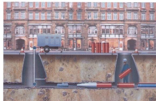
Pipe bursting (dynamic/static)
