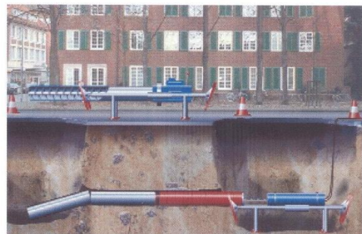
Directional drilling method
