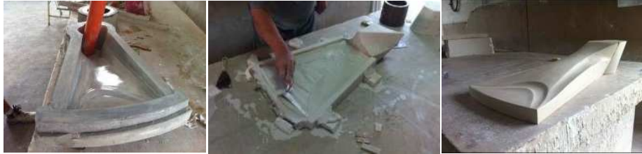
FIG. 21. 22 and 23. Re-composed Stereotomy Workshop : Processing of the step
