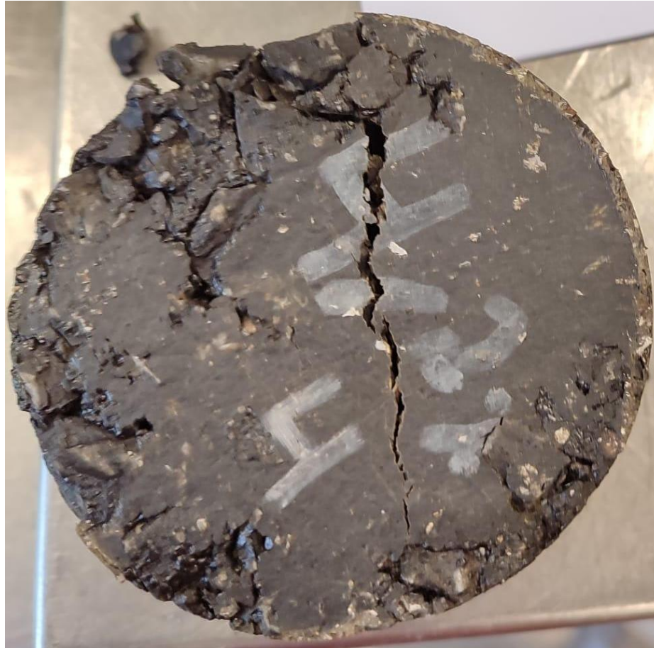
Figure A.20.4 - Specimen 4 - Type of failure
