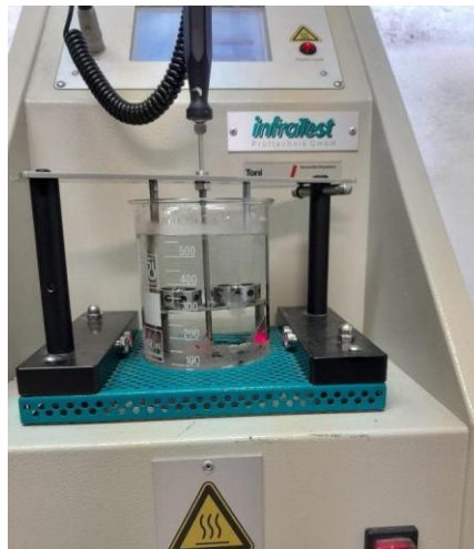
Figure 3.3 - Softening temperature by ring and ball test
