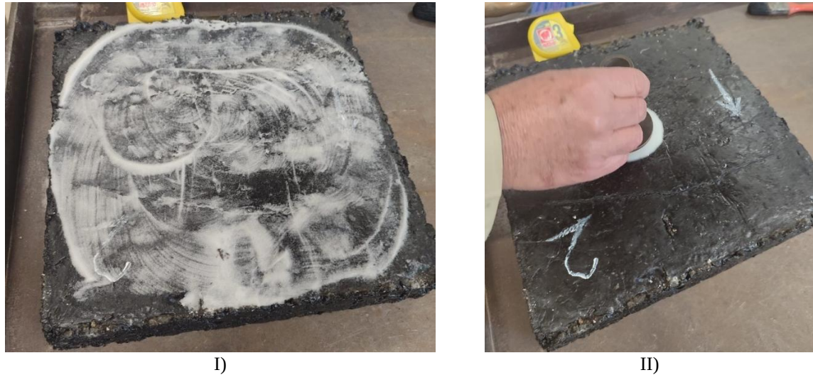
Figure 4.8- I) Insufficient surface to spread the glass spheres; II) Smoothness and lack of irregularities in the slab
