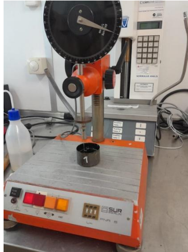
Figure 3.4 - Penetration test equipment
