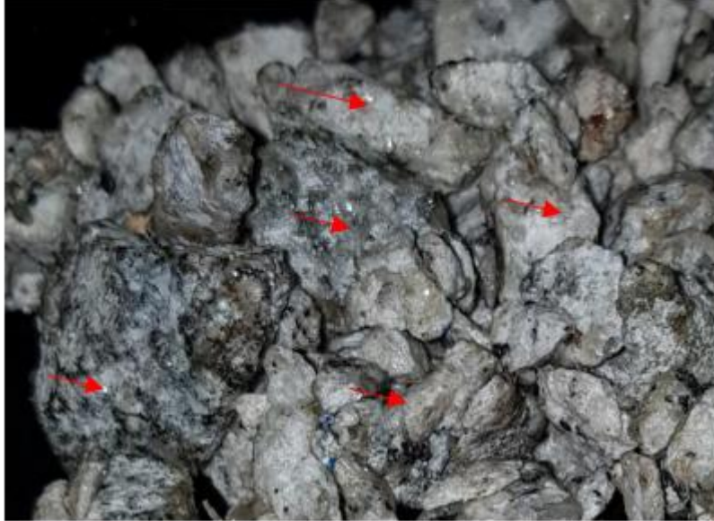
Figure 2.8 - Aggregate coated with plastic (Radeef et al., 2022)
