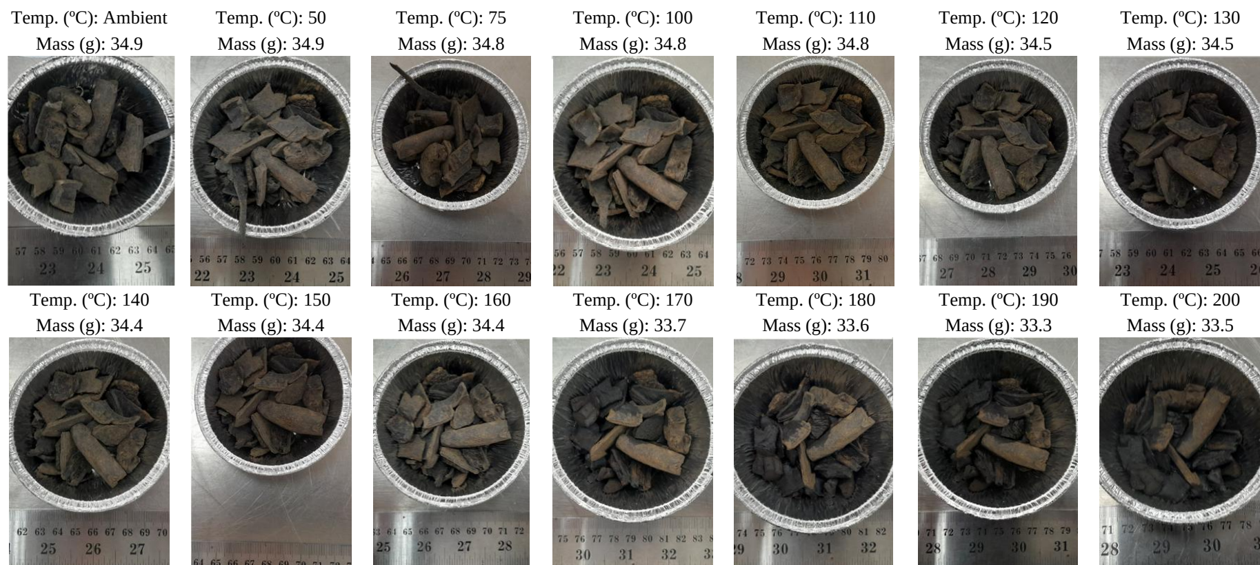
Figure A.3.16 - Sample A – Non floating black plastic
