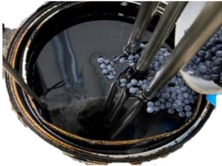
Figure 2.9 - Mixture between bitumen and plastic pellets (Giustozzi et al., 2022)
