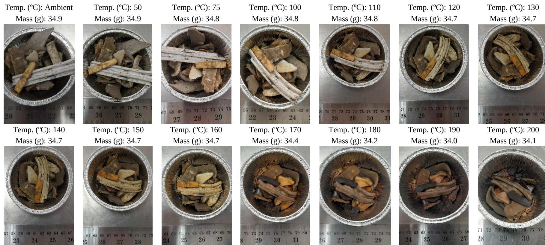
Figure A.3.14 - Sample A – Non floating white plastics
