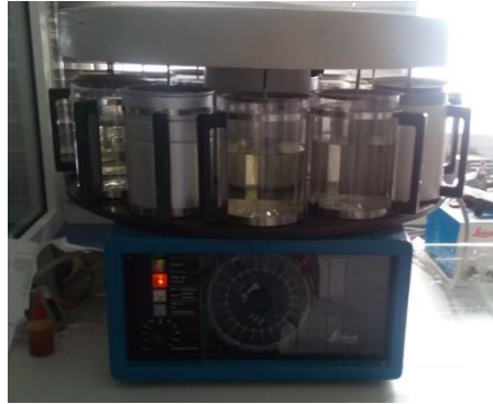
Figure 8. Automated tissue processor.
